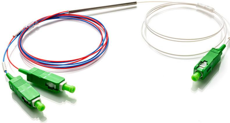
The Whyte range of mini optical taps operate over a wide range of optical wavelengths from 1260 to 1650nm featuring low insertion loss, high uniformity across output ports, high return loss and excellent directivity performance. These taps are terminated with SC/APC male connectors.
