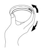
(7) When sensor unit is locked, tighten the locking screw.
