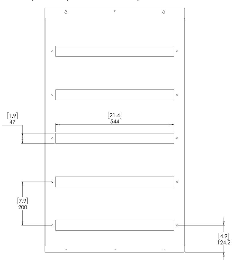
COVER PANEL CONFIGURATIONS SLOT SIZES 157, 228, 319, 371 & 458mm. ALLOWS FOR NEAT FINISHING WITH DIFFERENT SET UPS OF BREAKER AND MODULES
