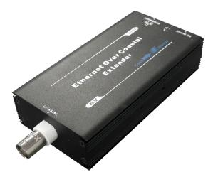
The DTV-IPCOAX/R is Ethernet and power signal receiver over single coaxial cable. The DTV-IPCOAX/R is used with DTV-IPCOAX/T, which is an ideal solution for reconstruction of old projects without any change of existing coaxial cable. You needn't change coax into network cable when you want to change analog cameras into IP cameras. Both of Ethernet and power transmission distance reach max up to 1000 meters.
