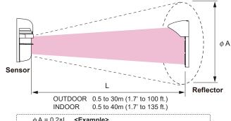
$\phi$  A = 0.2×L **<Example>**L = 10m (33') :  $\phi$  A =  $\phi$  2.0m (6.6')
