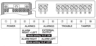
POWER : 9 to 28V DC (non-polarity) Current consumption 30mA max. ALARM OUTPUT (1): N.C./N.O. selectable, 30V (AC/DC) 0.2A max. (Resistive load) ALARM OUTPUT (2): N.C./N.O. selectable, 30V (AC/DC) 0.2A max. (Resistive load)
