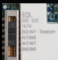
Built in EOL resistors
