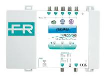
5-input (B1+FM, 4x VHF/UHF flexible) programmable headend to carry out high selectivity filters with up to 118dBµV output level for each filter. 32 filters from 1 to 6 channels, each with 9 selectivity levels.
